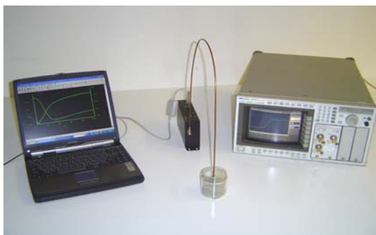
Dr. Hager's research setup for monitoring cement cure
