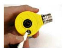
With CoreTech™, the activation of the zero set feature via set line or push button assigns the zero pulse to the current encoder position (adjusted to the rising edge of the A channel). No mechanical detachment or rotation of the encoder is necessary. This saves important time for service personnel.
