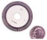
Unlike conventional code disks with a continuous repetition of opaque and transparent fields, the very small CoreTech™ disk condenses absolute position information into one non-repeating circular barcode pattern. A second track with 1024 analog sin/cos cycles is used to enhance resolution and accuracy.
