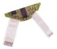
In order to find a solution to this dilemma, Stegmann has created the new CoreTech<sup>TM</sup> encoder generation. Core modules, which use an identical *Custom-designed High-Scale Hybrid OPTO-ASIC*, are the heart of all incremental and absolute CoreTech<sup>TM</sup> encoders.
