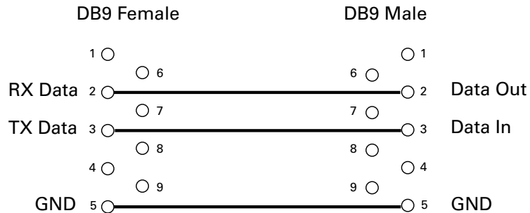
FIGURE 53. RS232 extension cable/connector wiring diagram
