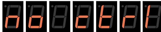
FIGURE 46. "No control" message will scroll when no valid radio signal is present
